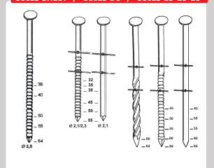
COILS SHEET 35 - 64 mm Ø 2,5 mm
